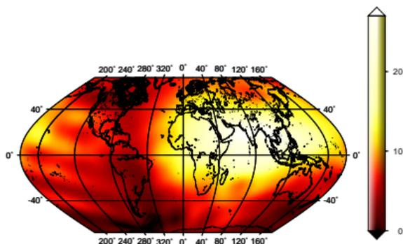
Example of ionospheric TEC (in TECU,  $10^{16} \text{ e}^-/\text{m}^2$ ). From a combination of GPS, altimetry, and COSMIC data, 21/7 2007 9:00 UTC. From M. Alizadeh.
