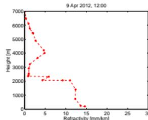
Examples of vertical profiles of the wet refractivity. From Wien/Hohe Warte radiosonde data.
