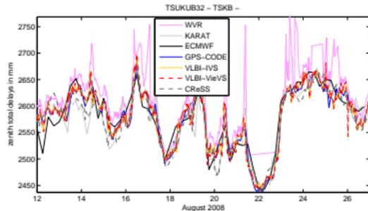
Comparison of tropospheric delays estimated using different techniques during the CONT08 campaign (12-26 August, 2008); from Teke et al. [2011].
