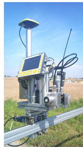
Fig. 7: MOBA rail-bound test robot
