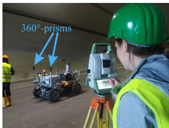
Fig. 5. Picture of how reference trajectory was obtained. Photo by Disaster Competence Network Austria (DCNA).
